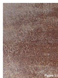
Conservation of works: Figure 11. Detail of a Corten steel work before restoration, with a dirty surface and limescale residues. Figure 12. Cleaning of the surface and application of protective coatings, to protect against excess moisture. Figure 13. Students from the Degree in Heritage Conservation, on learning practices for the works restoration.
